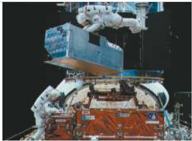
Installation of COSTAR to fix Hubble's vision. SMI.
