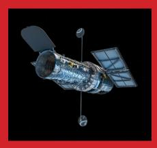
**Dimensions:** Length: 13.2 metres, diameter: 4.2 metres. In addition two solar panels each of which are 2.45 x 7.56 metres.
