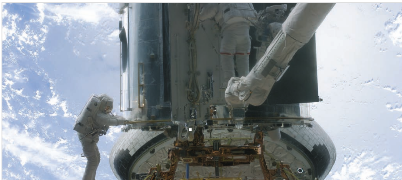
Fig 3: The external radiator for the NICMOS cooling system being put in place by the astronauts during SM3B.
