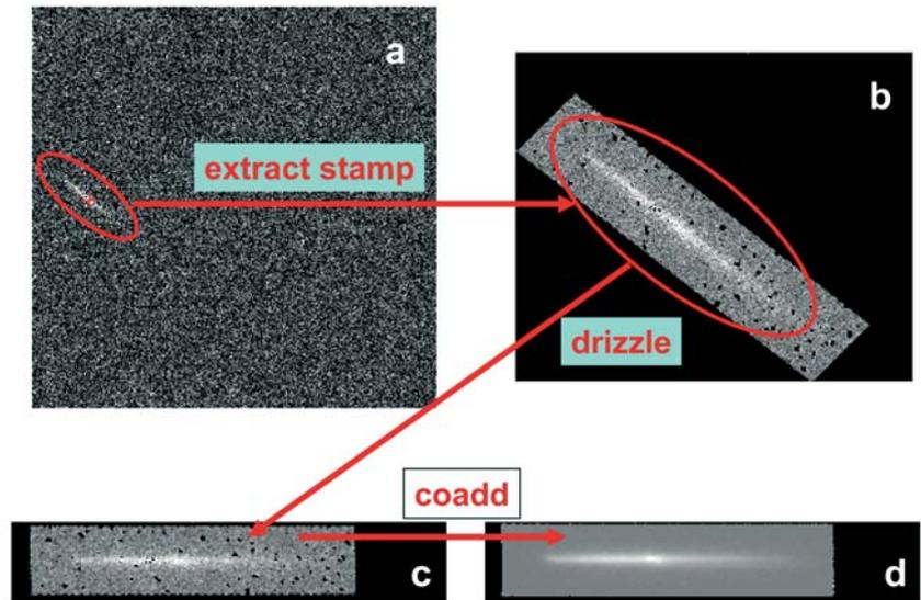
**Fig 2:** aXedrizzle: the object marked in panel a is extracted as a stamp image (b). The stamp image is drizzled to an image with constant dispersion and constant pixel scale in the cross dispersion direction (c). The deep 2D drizzled image (d) is then used to extract the 1D spectrum.
