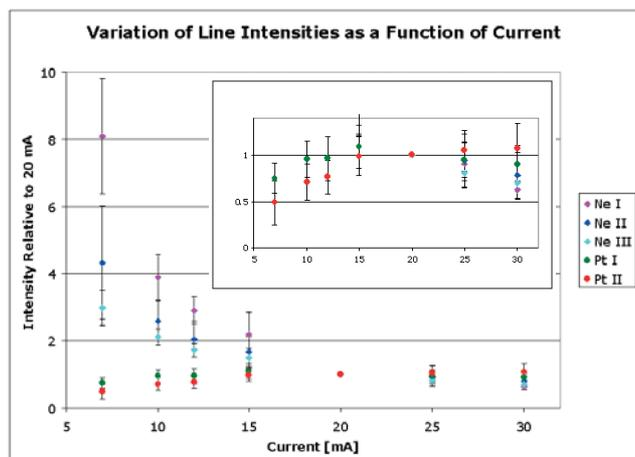
**Fig 2:** Variation of the line intensities as a function of the operating current of the lamp. The error bars represent uncertainty at the one standard deviation level. Spectra were taken at 7, 10, 12, 15, 20, 25 and 30 mA. Note the pronounced difference in the behaviour of the gas and metal (inset) lines.
