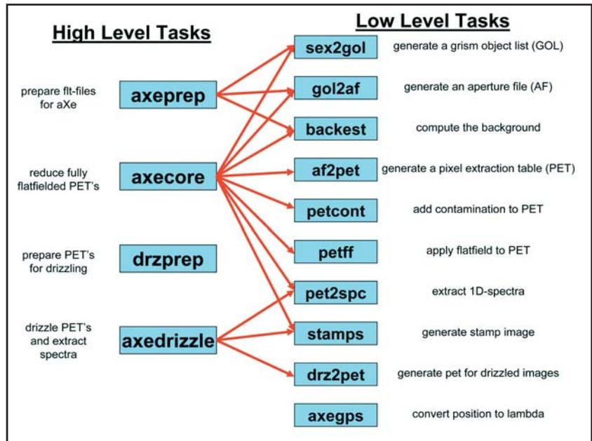
**Fig 1:** Overview of all aXe 1.4 tasks. The arrows indicate the interactions between the High Level and Low Level Tasks.
