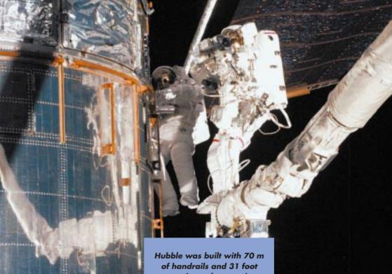
During each EVA one astronaut (known as EVA1) accomplishes primarily the free-floating portions of the EVA tasks while the other astronaut (EVA2) works from a special platform attached to the Shuttle's robotic arm.
